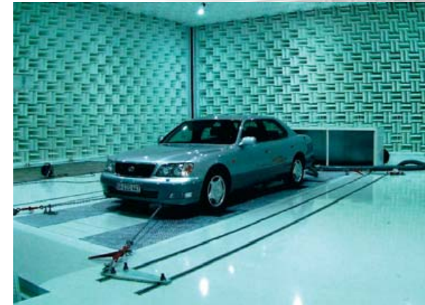
SAL Sassenburg, ASONAD-S, f_g = 63 Hz, 20 x 17 x 6 m (Schaumstoffkeile)
