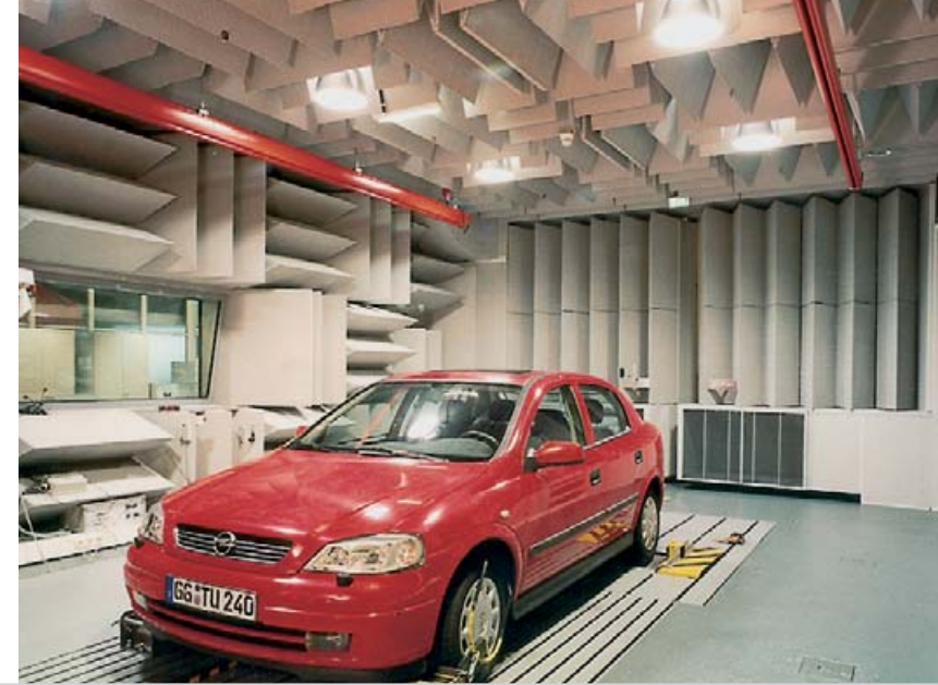
Opel AG f_g = 100 \text{ Hz} L \times B \times H = 10 \times 6 \times 4 \text{ m} ASONAD-ML (Lochblechabdeckung)
